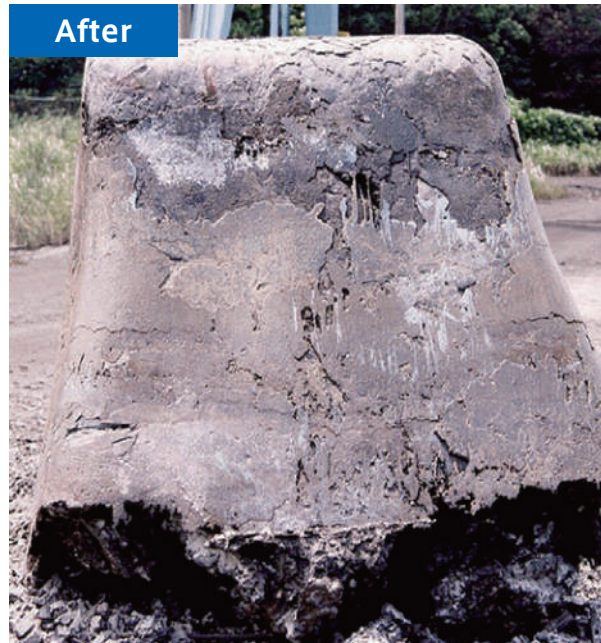
Slag with KAILEX (before crushed)
